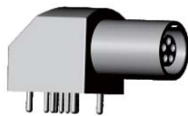
RM-EPG Elbow (90°) Receptacle for printed circuit, key (G) or keys(A..F) (solder or screw fixing)
