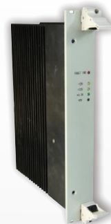
Standard 6U Package Size (mm: 233x160x40)
